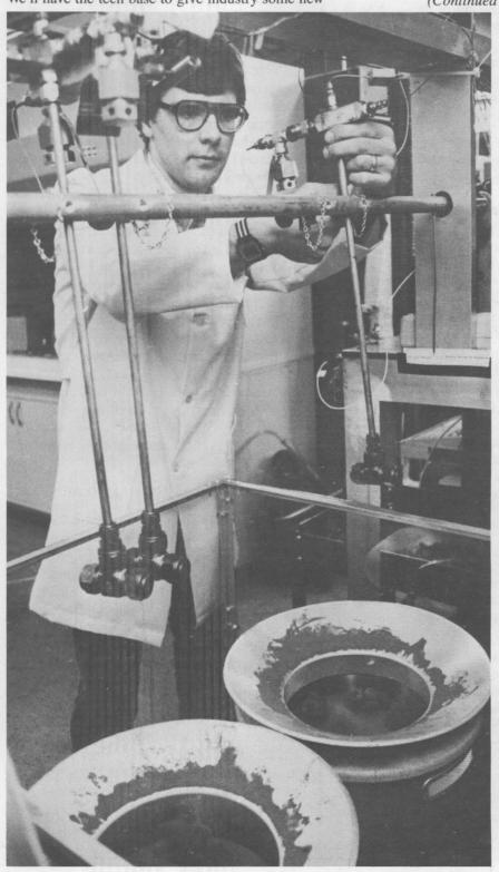
RICH KOTTENSTETTE (6212) prepares reactor chambers (35cc volume) containing coal, coal solvent, a catalyst, and high-pressure hydrogen for insertion into hot (400°C) sand in coal-liquefaction experiment.
